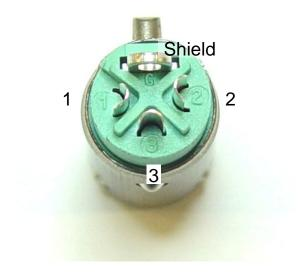
Vibration pickup connector, solder-side view
